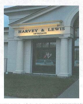
PIN LETTER SIGNS with SINGLE BULB REFLECTIVE UPLIGHTING Upscale design with no spillage above "canopy"
